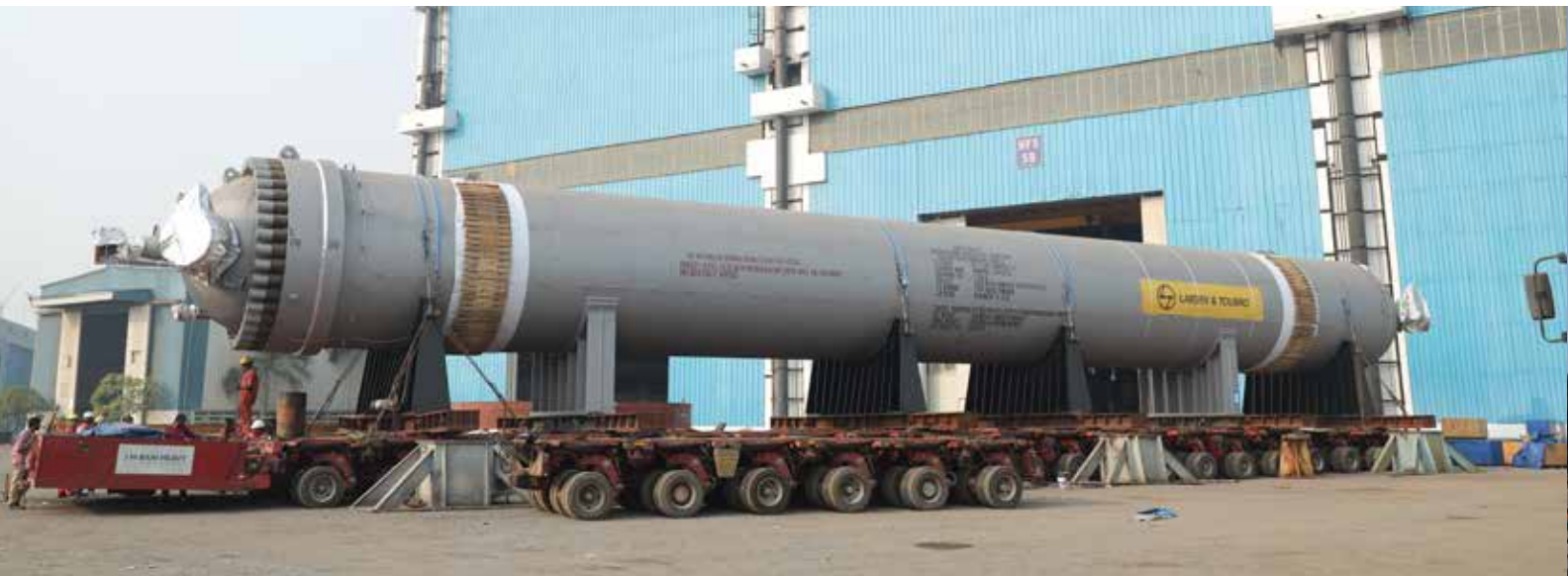
Ammonia Converter and Basket for OCI Beaumont, USA
